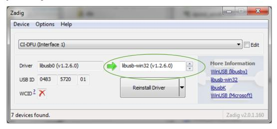
Click *Install Driver* to proceed installing libusb driver. This could take up to 1 minute to complete.
