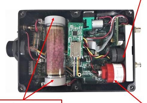
Step 8: Apply force to both ends, gently push new Filter tube into connectors
