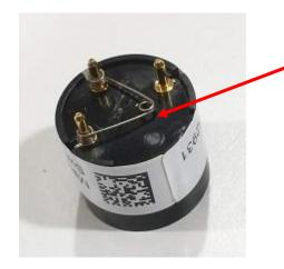
Step **5**: remove short-cutting spring from new C2H4 sensor. (the spring keeps sensor from sensitivity/baseline drift during storage. Save it later for your old sensor)
