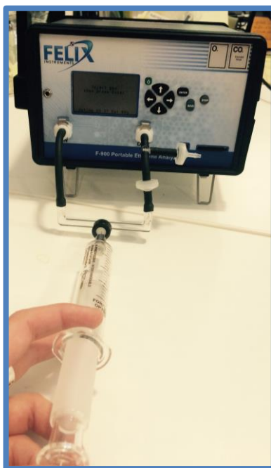
Figure 13: GC Emulation port connected to front of instrument for small volume samples.
