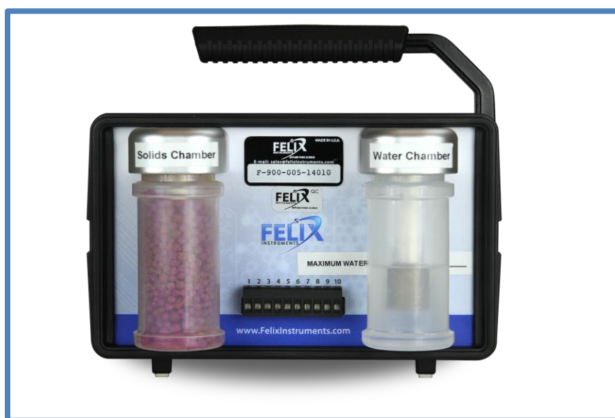
Figure 21: Solids Chamber and Water Chamber on back of instrument.
