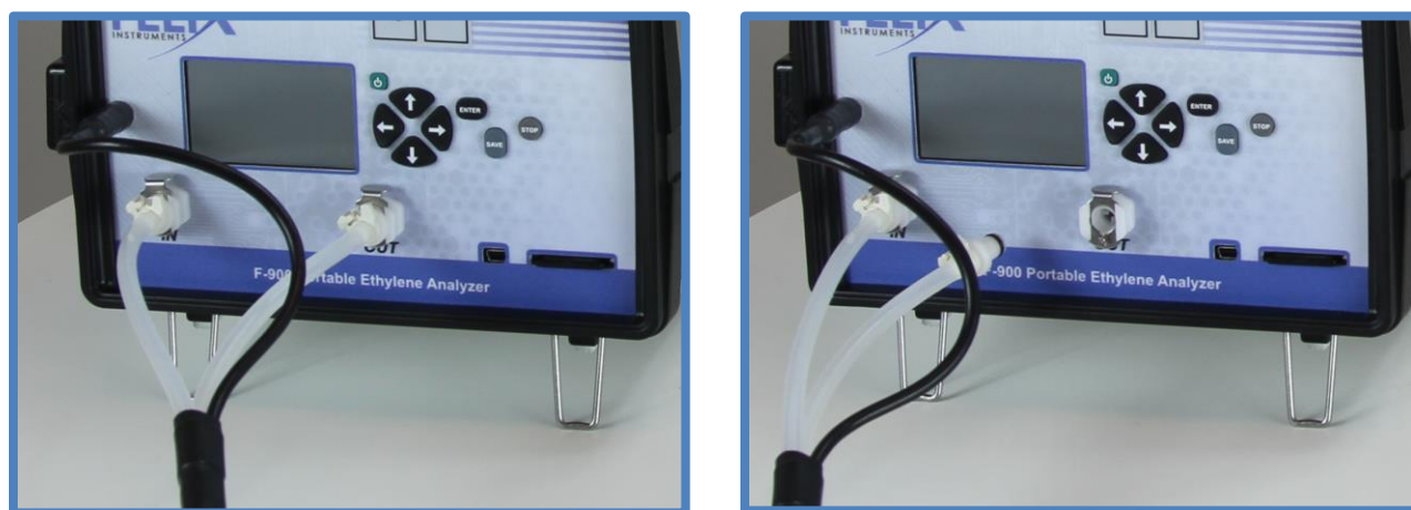
Figure 12: Using conditioned air to replenish the fruit chamber by connecting the IN and the OUT (left); using ambient air to replenish the fruit chamber by disconnecting the OUT (right).
