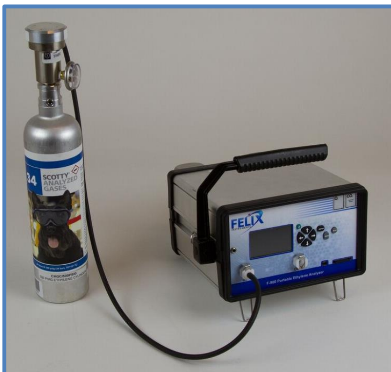
Figure 17: Ethylene calibration gas cylinder with On Demand Flow Regulator connected to F-900 IN port.
