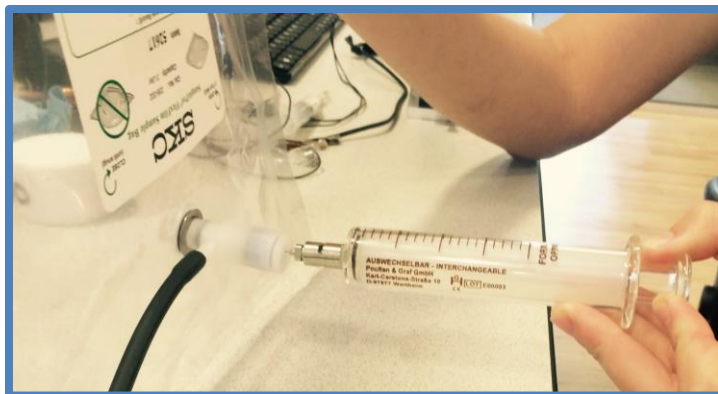
Figure 16: Proper technique for filling glass syringe from sample bag for GC Emulation Mode.
