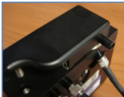
Figure 10: Fiber-optic attached to the side of the CI-710 for Reflectance mode.
