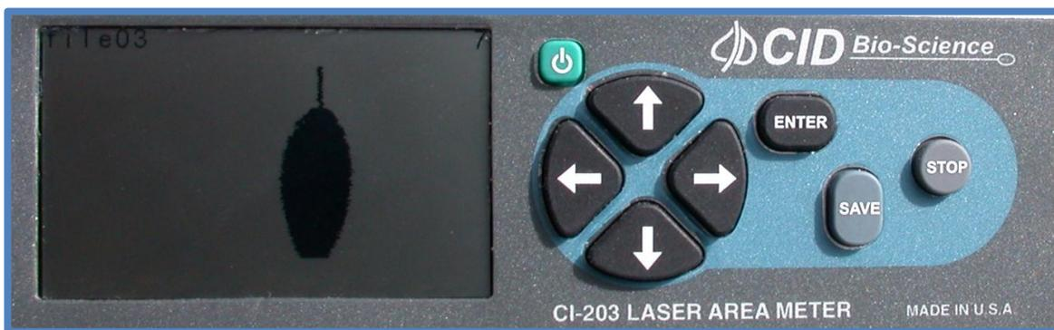
Figure 4. Image of measured leaf on CI-203 display screen
