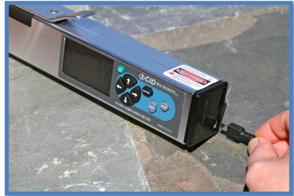
Figure 6. SDcard and USB cable connection for CI-203
