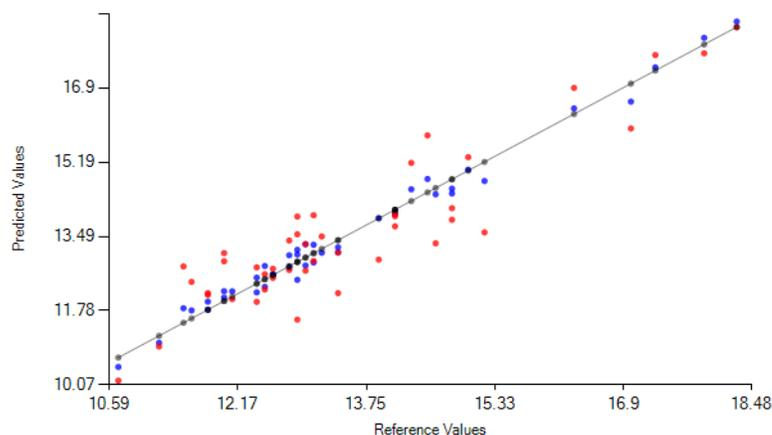
Figure 2. Prediction error for pears using the F-750. Specimen most strongly correlated to the calculated trend line show the greatest accuracy of prediction (Red; Cross validation Prediction, Blue; Training set prediction).
